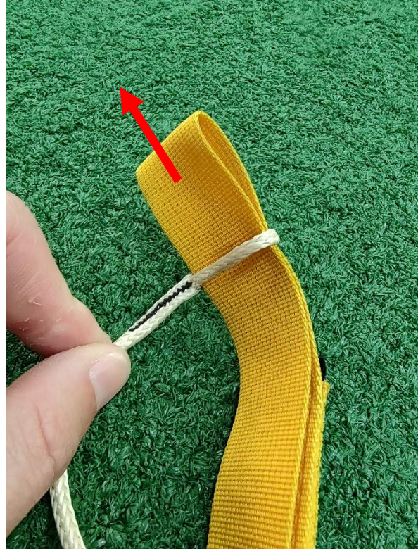
Figure 2.10 Route the handle of the toggle through the loop end of the steering line.
