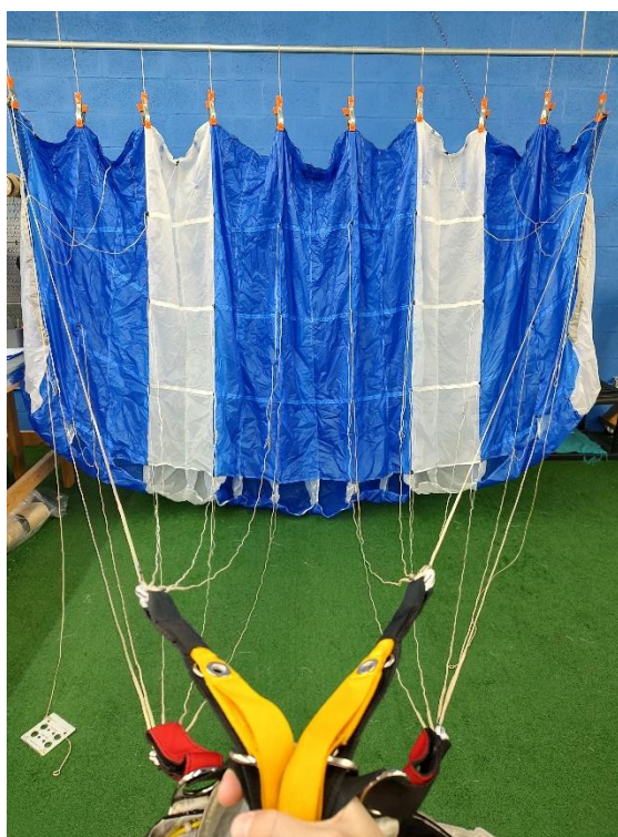
Figure 2.4 Suspension lines attached to risers.
