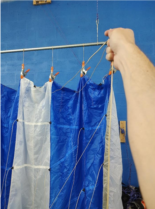
Figure 2.5 Upper steering lines are clear of suspension lines.
