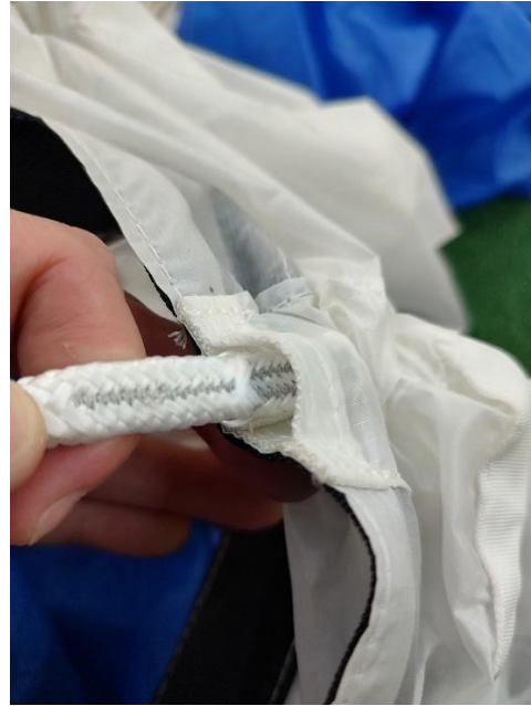
Figure 2.14 Insert the locking tab into the channel.
