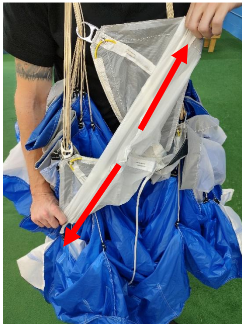
Figure 2.15 Pull collapse cable back into the slider.
