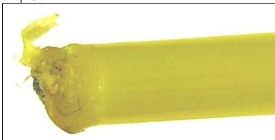
Examples of poorly burned cable ends.
