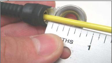
Begin measuring where the cable comes out of the end fitting.
