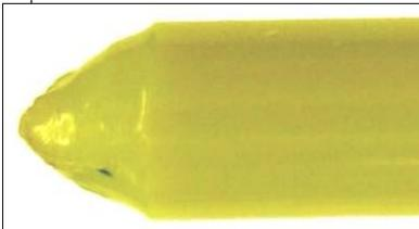
An example of a perfectly burned and smoothed end after being heated only one time.
