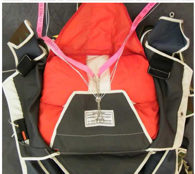
Drisse provisoire Temporary bridle
