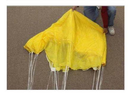
Fold the C lines to the left, past the B line path as far as possible, than bring them back and lay the C lines on top of the B lines. This results in the canopy fabric between the B and C lines being folded on the left side of the canopy and the C lines are directly on top of the B lines. Straighten this fold as necessary.
