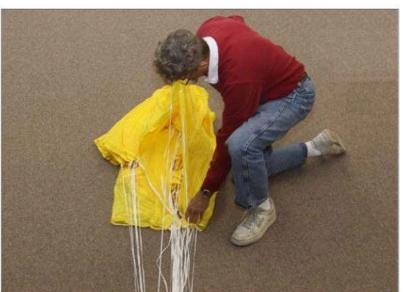
Fold the tail on each side maintaining the steering lines on top of the other lines.
