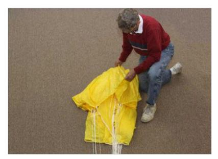
Look up the lines to all the line attachement points. All lines should go up to the attachment points with no canopy fabric between them.
