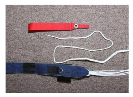
2. Feed the steering line through the ring on the riser.
