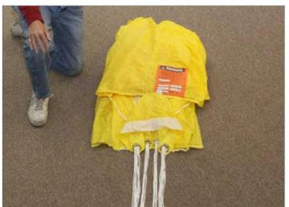
Grasp the tail at each edge of the center cell and pull down until it is even with the lower edge of the folded canopy. Raise the center cell of the tail six inches and inspect the D lines and steering lines. Make sure all lines are taut.
