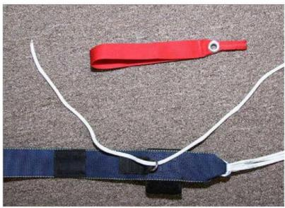
3. Feed the steering line through the grommet in the toggle, around the toggle and back through the grommet.
