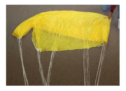
Hold down the canopy at the A line path, find the seven "T" seams directly above the B line path and fold to the left, placing the B lines on top of the A lines.
