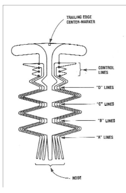
Hold the canopy parallel to the floor with the nose facing down. Hold the lines in one hand while using your free arm to support the canopy fabric. While maintaining even tension on the lines, gently place the canopy back down on the floor or packing table with the nose facing down.
