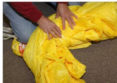
A dimple should be made between the left and right line groups below the slider
