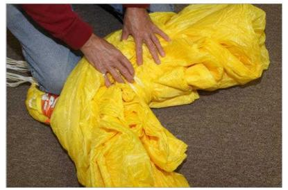
c) In case of a two pin center line configuration, a dimple should also be made between the left and right line groups below the slider.
