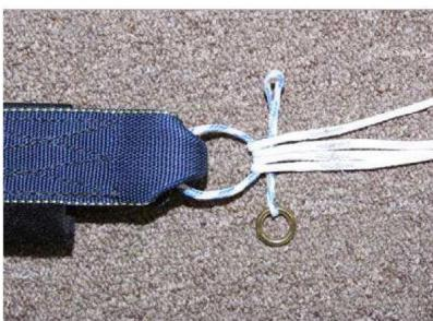
3. Feed the loop end of the link through the riser again, second time.
