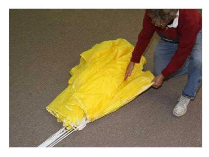
Flake material between the A and B lines away from the line channel in the center of the pack job. Be sure that all three "T" seams to the right of the center cell are neatly flaked.
