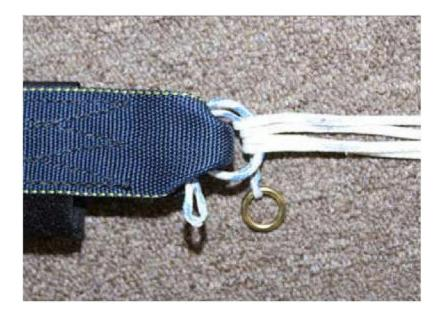
4. Feed the loop end of the link through the lines again, third time.
