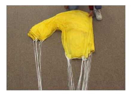
Grasp the seven "T" seams directly above the D line path and fold to the left placing the D lines on top of the C line path. The material between the C and D lines should be folded to the right of the lines.
