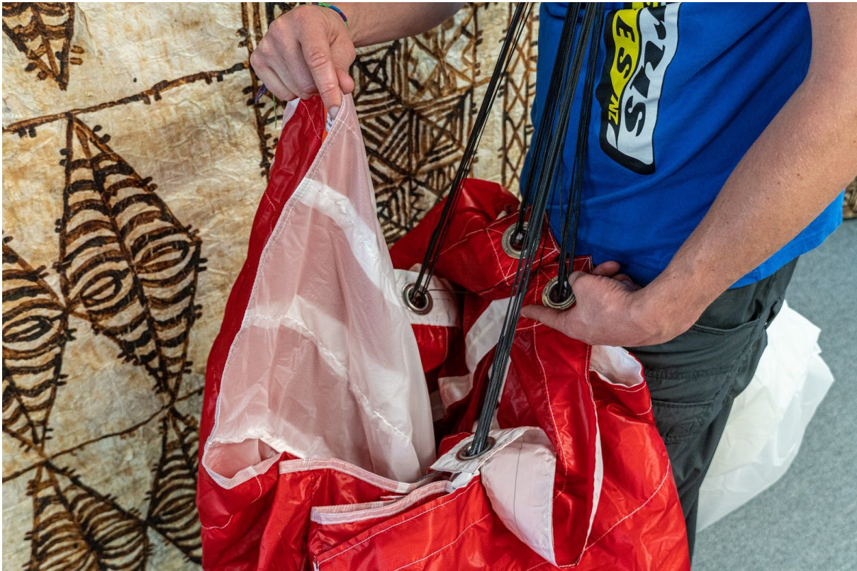
Tail lifted to high past grommets
