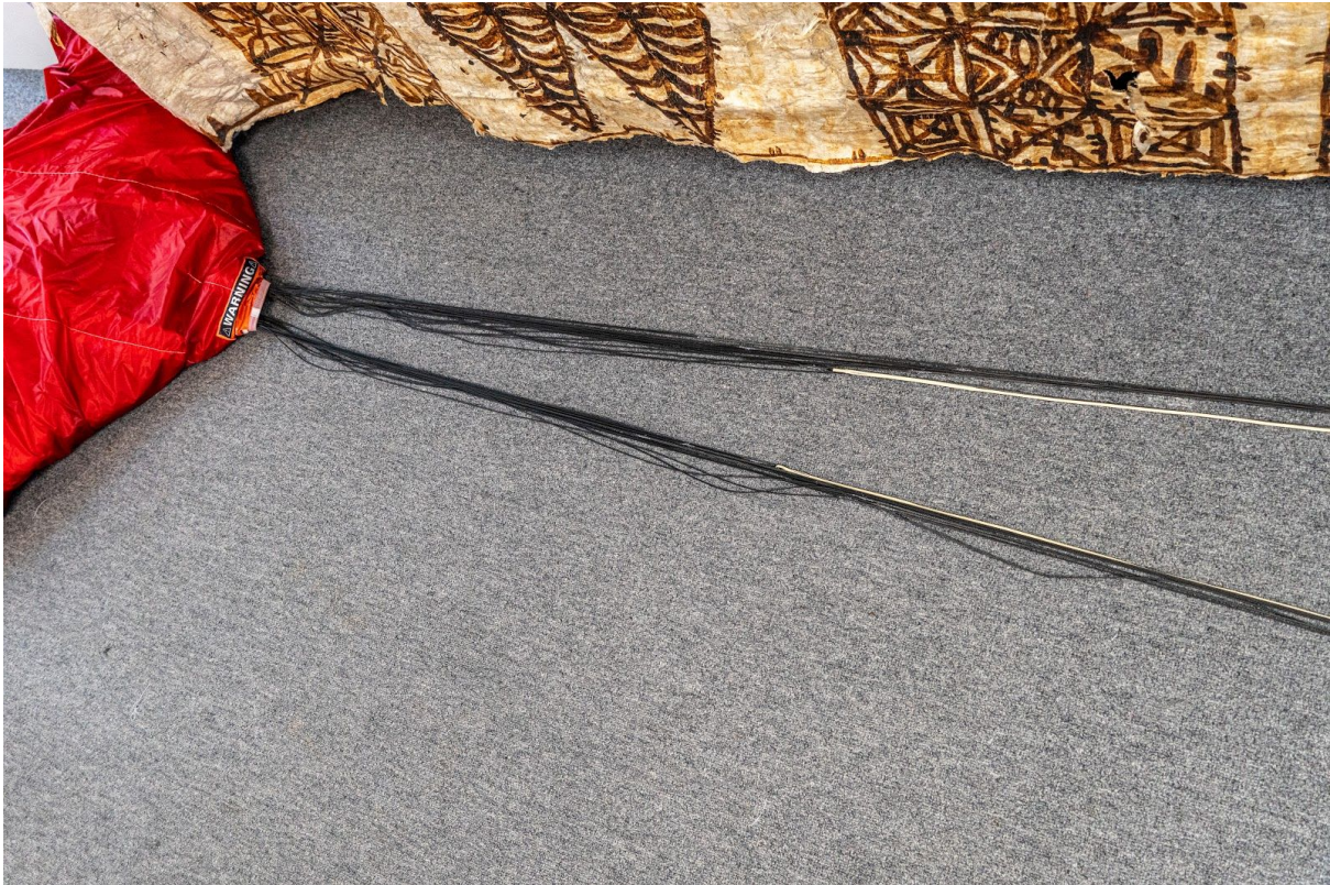
Manageable slack that can be distributed safely and evenly through line stows
