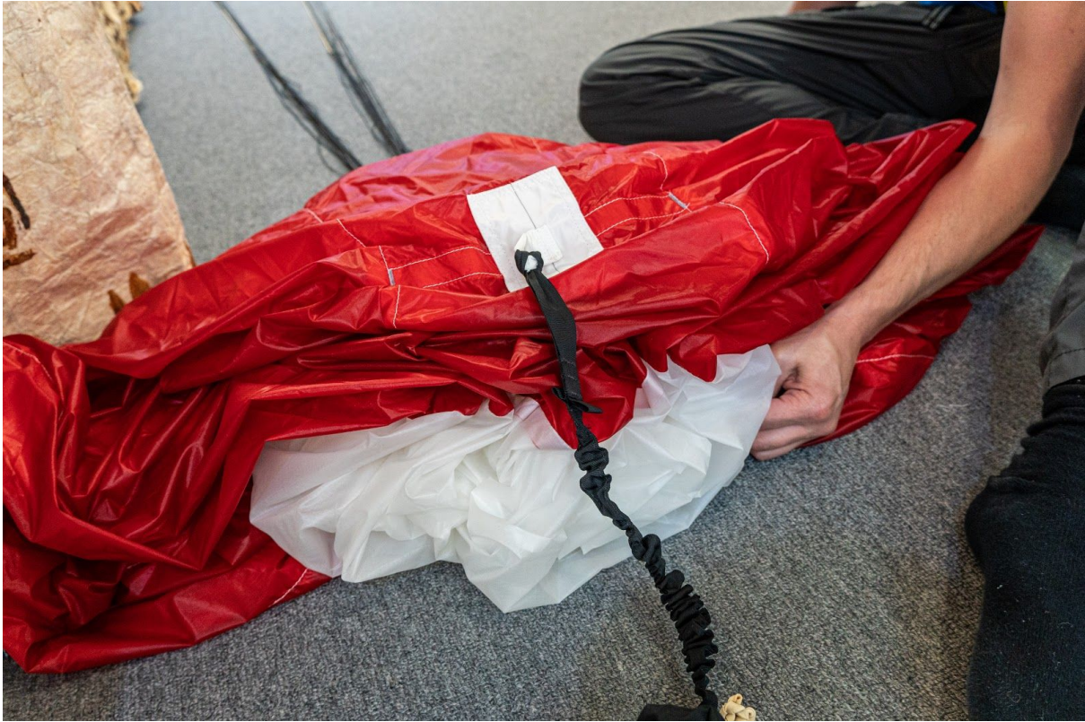
Pulling top skin to tidy line slack. Be careful not to pull excessively, it can result in increasing the problem.
