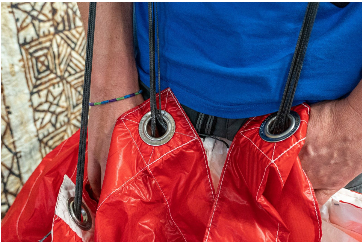
Correct tension with no loose lines
