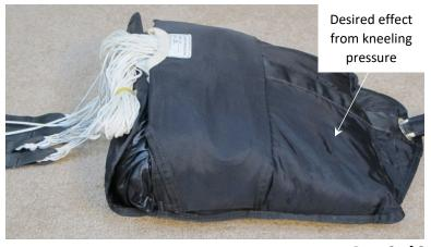
**Step 9.** Flip main bag into container rotating 180 degrees. Line stows should be facing the reserve tray as shown. →
