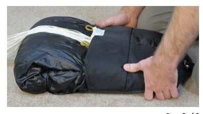
**Step 6.** Stand D-bag up, fold/roll remaining canopy fabric into bag as shown.  $\downarrow \rightarrow$
