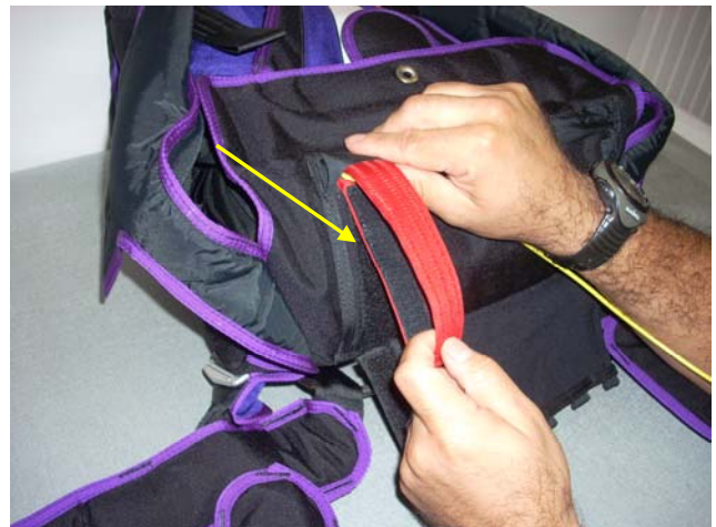
Begin by mating the Hook Velcro of the AFF Left Side Main Deployment Handle with the Pile Velcro on the Main Container Bottom Flap.
