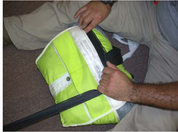
Alternate back and forth until lines are into the pocket and Reserve Risers are to the Free-bag.
