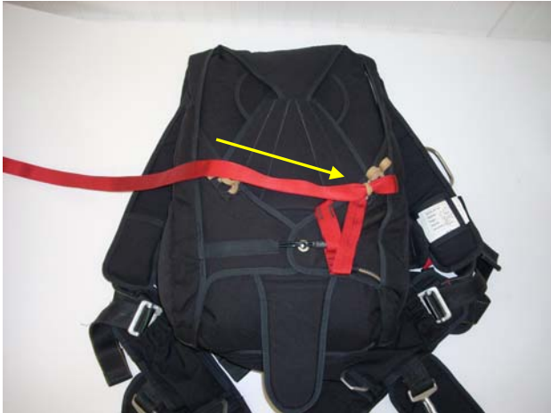
Stow the first bight of the Static Line into the first rubber band.
