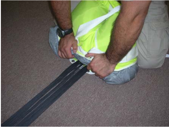
Fold the Free-bag over the canopy in order to close with the safety stow.
