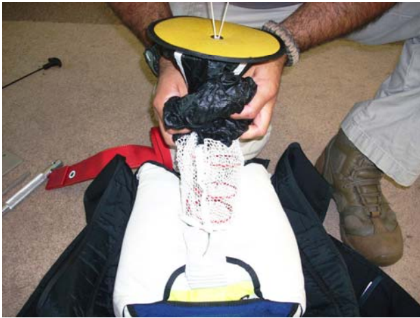
Center the Pilot-chute over the Side Flap grommets.
