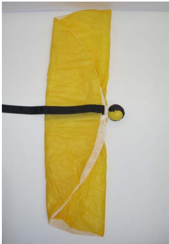
Fold the Pilot chute in 1/2 again with the bridle still coming out of the middle.
