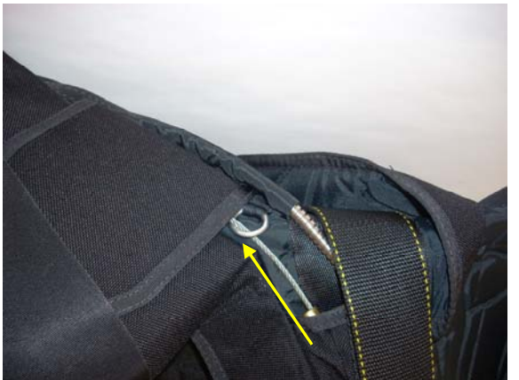
Open up the Reserve Container. Check to be sure that the Reserve Ripcord is installed correctly.
