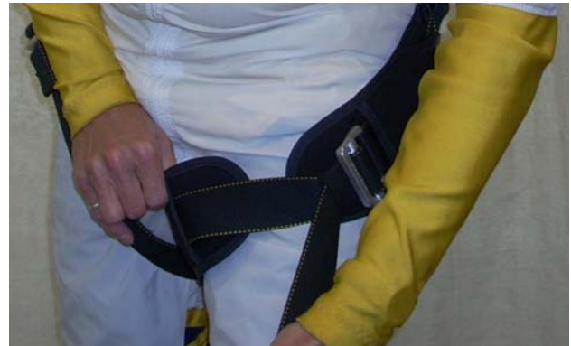
Adjusting the Leg Straps.
