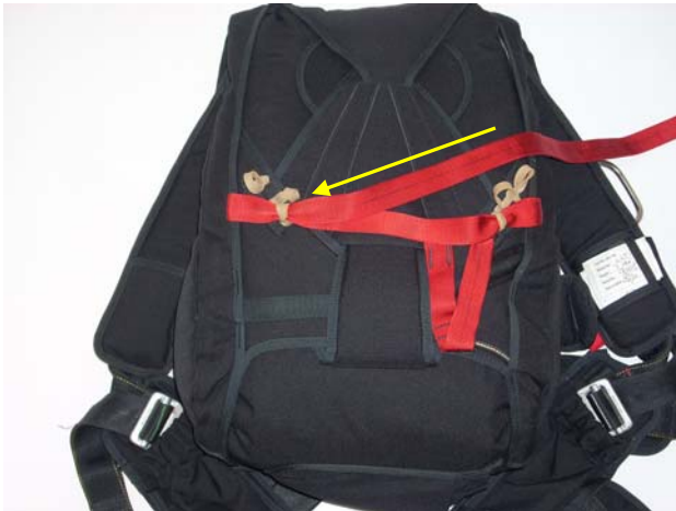
Stow the second bight of the Static Line into the opposite side rubber band.
