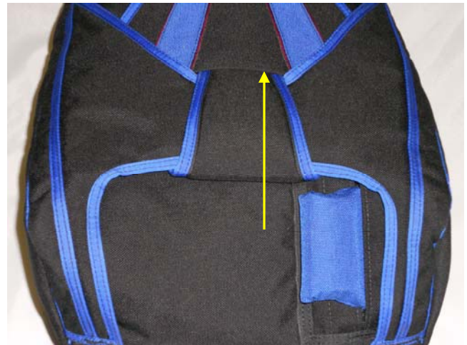
Close the Main Pin Protector Flap.
