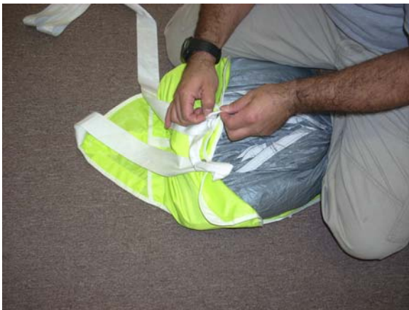
Use the Free-bag bridle to hold the safety stow in place.
