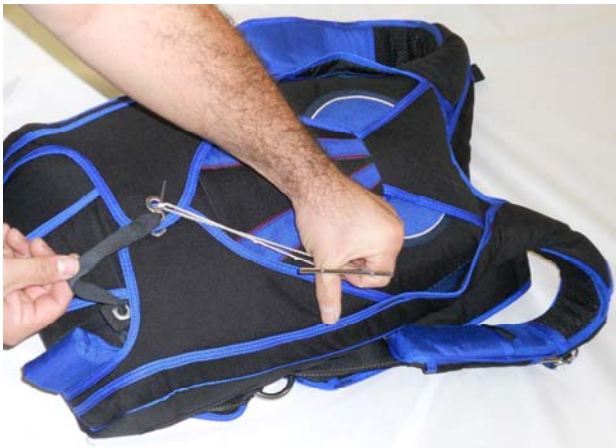
Close the Left Side Flap and secure with the Straight Pin.
