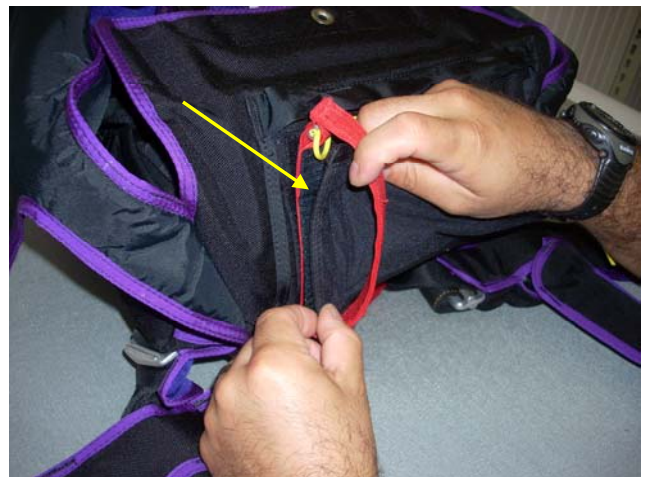
Mate the Pile Velcro of the Pouch to the Hook Velcro of the AFF Left Side Handle.
