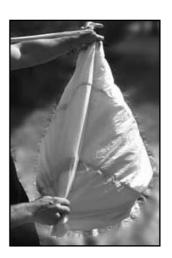
At this point, your canopy must look like a roll. Swing it out slightly so that the lines stay taut and gently lay it on the floor. Beware to maintain tension on lines.
