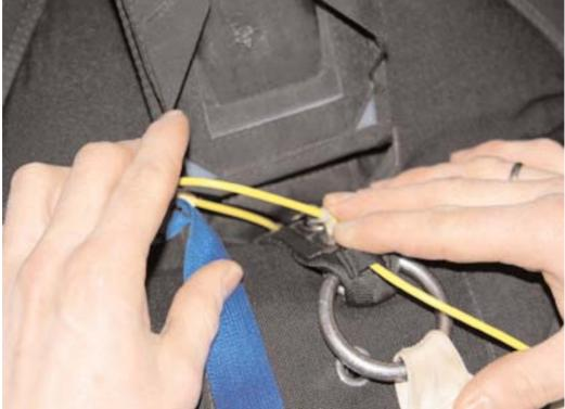
Then route the Drogue release cable through the Drogue release loop from the Drogue riser.
