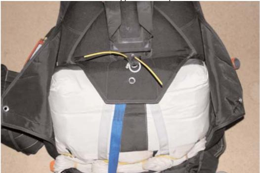
Connect the Drogue chute. The Drogue chute release cable (left on the shot), must be prepared without being running into the Drogue chute riser connecting loop.
