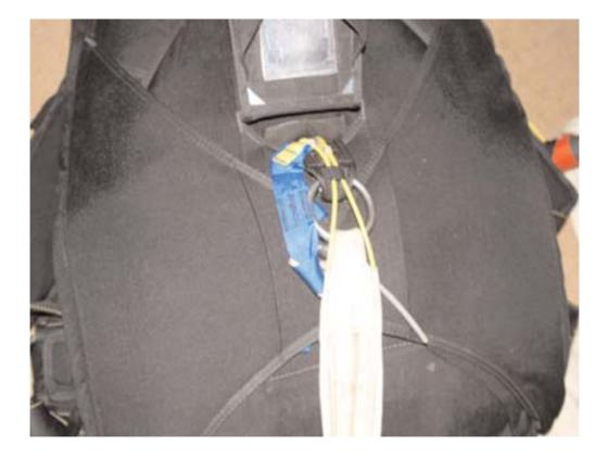
Stow the Drogue chute bridle under the main right flap toward the Drogue pouch. This process make sure that the main bag connecting bridle is on one side and the Drogue chute bridle is on the other side. This avoid any potential conflict between both bridles which can be caught by each other. Such conflict can pull the closing pin cable when the Drogue chute is jettisoned.
