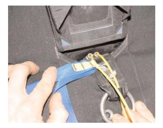
Stow the main Drogue release cable into its tunnel.
