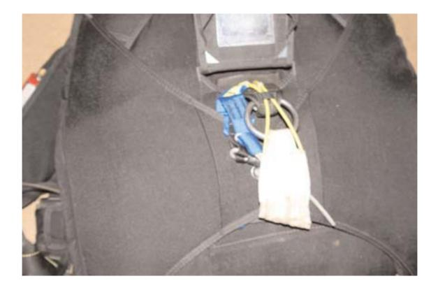
Stow the Drogue Chute in its pouch and close the main protecting flap.
