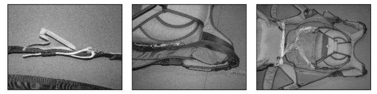
Lay the risers between the sides of the reserve container and the risers covers. Close the risers covers and stow the risers straight on the side of the reserve container.
