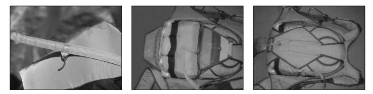
Pilot chute bridle must be route out toward the upper right side. Closing flap order is: -Bottom -Up -Left -Right
