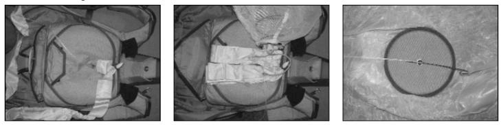
Fold or roll the pilot chute fabric at the top of the pilot chute parallel with the top of the container, and push this roll under the top plate of the pilot chute. Stow the remaining of the pilot chute fabric down the sides of the pilot chute top plate. Push the excess fabric under the pilot chute top plate. Fan out the pilot chute fabric excess, so that it extends wider than the bottom flap.
