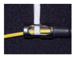
Routing of the white loop through the riser's grommet. Running of the white loop through one of the little round window.
