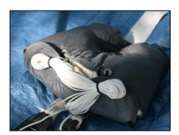
Leave a slack of 40 cm from the free bag to the risers. Remove the strips of loop velcro and mate the velcro at the mouth of the pouch, making sure that none of the suspension lines are trapped by the closure.
