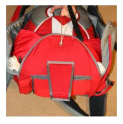
Pilot chute bridle must be route out toward the upper right side. Closing flap order is: -Bottom -Up -Left -Right
