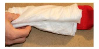
Tuck the slack of bridle into the pouch, then tuck the pilot chute. Spread widely the pilot chute into the pouch.
