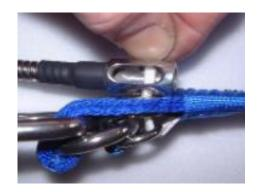
Fit the cable through the white loop and stow the remaining cable. Assembly must be done like on this photo.
