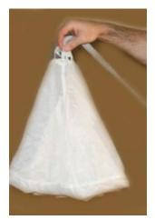
Set the main bag into the container with the line stows oriented toward the bottom. This position is important; if the line are oriented toward the top, it may be more difficult for the pilot chute to extract the bag. Also, the lines can snag easily any part of the container.
