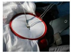
Compress the pilot chute and lock it with the temporary pin. Now pull all fabrics out from under the top plate so that the pilot chute fabric is spread out. At this point, check the lenght of the closing loop. If the pilot chute's top plate can rock back and forth or from side to side, the loop is too long. Shorten it so that when the pilot chute is compressed and locked with the temporary pin, the top plate is firmly seated in the nest formed by the shape of the free bag.
