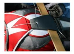
Close the top flap and secure it with the temporary pin.
