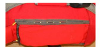
When pulling the handle both cables released and the pouch became free.
