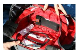
Slip the control unit into the back-pad and stowed it in its slot. Close the protecting flap. Installation is done. It is possible to install the control unit in the right ring cover (only available under request for student unit with adapted cable lenght).
