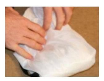
Put the pilot chute against the container with the bridle slack between the pilot chute and the pouch.
