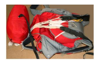
Lay the risers between the sides of the reserve container and the risers covers. Close the risers covers and stow the risers straight on the side of the reserve container.
