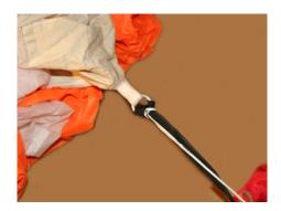
Run the steering line into the tape loop located under the pin setting.
