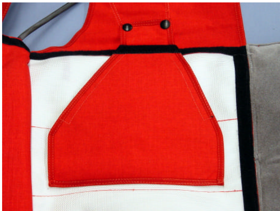
Fig 31 Ripcord pins in position
