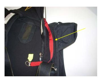
Mate the Pile Velcro of the RSL with the Hook Velcro under the RSL channel of the Left Side Reserve Riser. Start at the lower end of the channel and proceed to the top.
