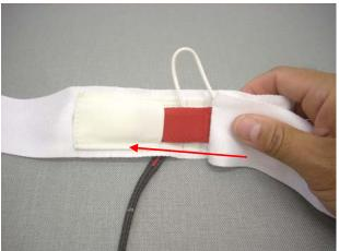
Tuck the stiffened T-III Tab into the tuck channel on top of the Long Pin Channel.
