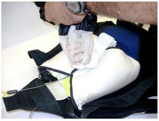
Thread a pull-up cord through the Reserve Pilot-chute and center over the side flap grommets.
