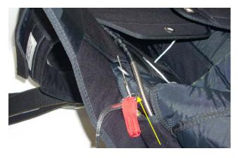
Pass the Ripcord Cable through the guide ring on the Container.
