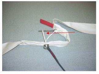
Slide the Long Pin through the loop then stow into the channel under the tuck tab flap. Be certain that it is in it's own channel.
