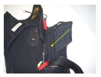
Close cover when Velcro has been mated and RSL has been installed.
