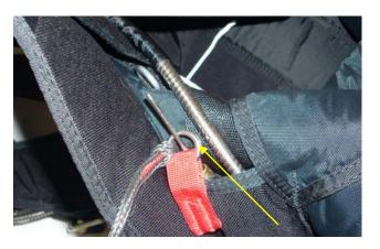
Pass the Ripcord Cable through the guide ring in the middle of the RSL.
