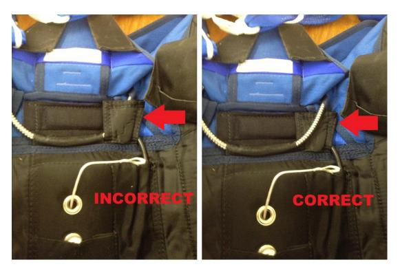
There is a pad that should be used to protect the cable for the AAD control unit from being damaged by the cutaway cable housing. Please reference the picture for proper use of this pad.
