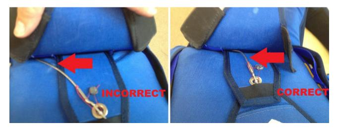
Make sure the reserve cable is routed IN BETWEEN the outer and inner reserve flaps, and NOT around the side. Please reference the picture for proper routing.
