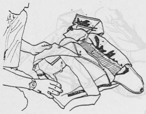
AB. Repeat folding procedure from previous side and tuck folded bridle under this side flap while making another 90 degree fold back to the center of the container.
