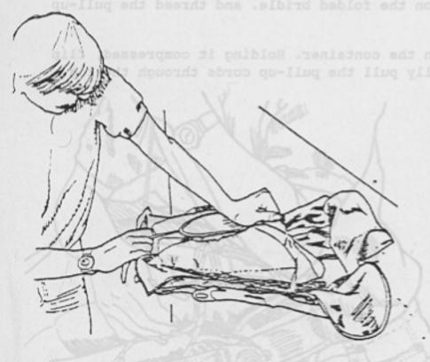
This is your opportunity to seat the pilot chute and adjust the pull force. The SST "Quick Loop" is designed to give the rigger the ability to do both of these things. Remember: 22 lb. to move the pin is all that is required.
