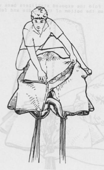
H. Fold each section of the nose outward from the center it takes air quickly during deployment.
