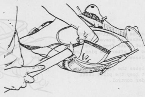
Using hemostats or needle nose pliers grip "Quick Loop" pull string about 1/4 inch back from edge of hat and push slack through hole in hat valance into area between top of pilot chute and bottom of hat.
