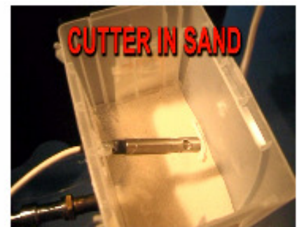
Cutter activation with loop and cutter severely contaminated with sand
