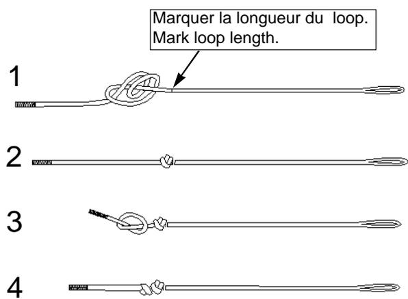
Be sure that both loops have the same length after tightening on the washer.
