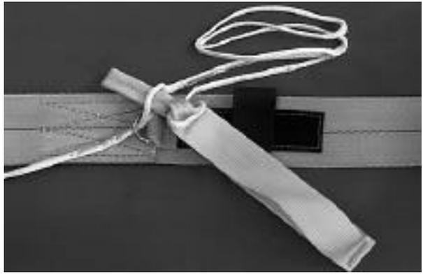
Stow line slack then secure it with the velcro fastener.
