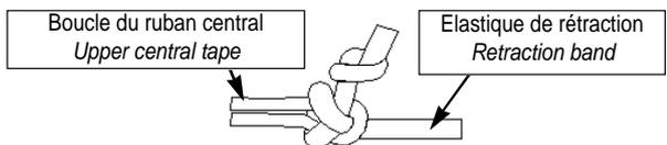
Simulate manually the pilot chute operation to secure the knot into the handle.
