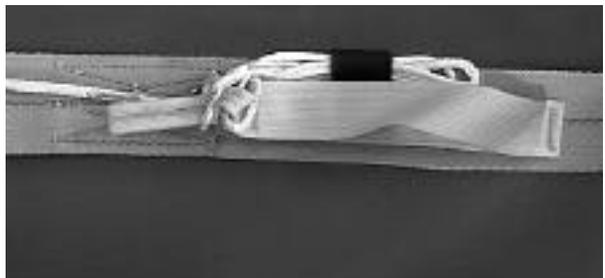
Reaching this stage of operations the reserve canopy is ready to be packed into the deployment bag according to the specific manual.
