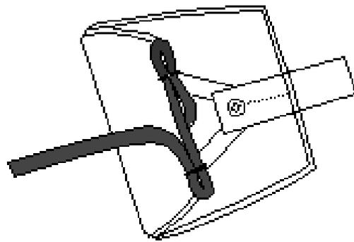
*If the harness-container is equipped with a FXC 12000 AOD it is advised to put less fabric into the left side of the bag. Roll over the bag without making twists and stow the lines into the cotton keepers.*
