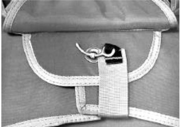
**Throw-away PC on leg strap (B version).** Mate the bridle onto the container velcro and slip bridle under right side flap.
